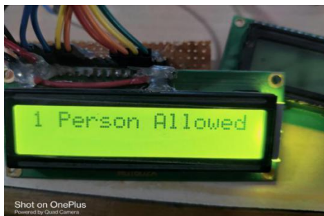
Fig.16. LCD displaying remaining persons that can allowed into room
